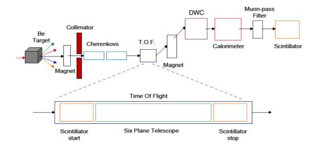
Fig. 1 – Schematic layout of the experiment.
